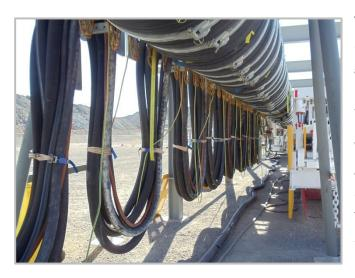
The Development Monorail system has proven to assist in the increase of advance rates within the maingate development unit, in a manner which greatly reduces the risk of personal injury and equipment wear and damage.
